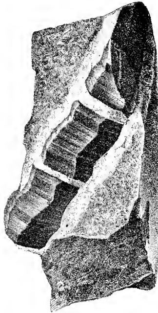
Fig. 22. Crystal of Corundum with its shell of cleared felspar forming the crystal "court" or crystal "compound."
